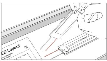
Remove the tape from the back of the LEDs and stick them in **ACM panel** according to the provided layout (refer to Figure 1 on page 2).
