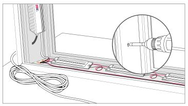
6 Drill holes on lightbox connect to the power supply.
