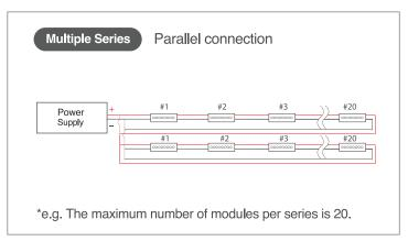
If you require **multiple modules**, they must be wired in parallel as a safe electrical operation mode. **Serial connection is not recommended**, as unbalanced voltage drops can lead to hazardous overload, potentially damaging the LED modules and causing uneven brightness.
